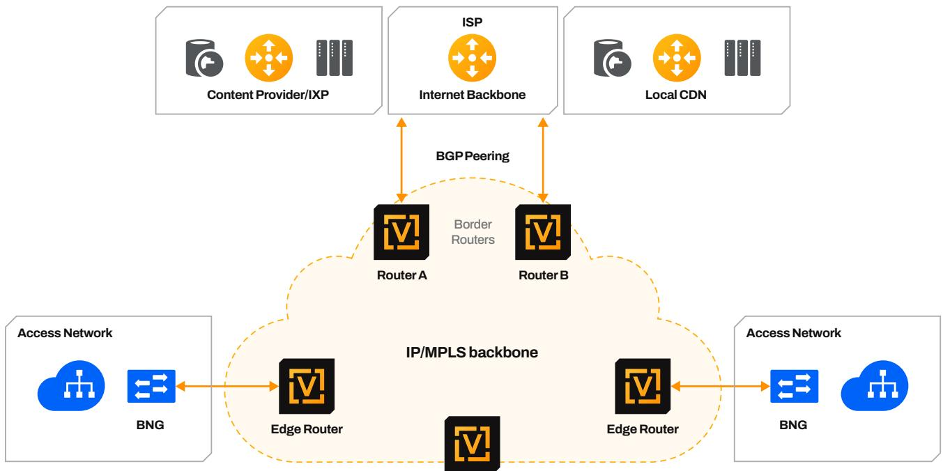
Understanding these critical challenges some points should be taken into consideration when choosing the right border routing platform to ensure it delivers crucial features and functions like support for a full internet routing table, RPKI, policies for filtering and traffic management, QoS, NAT, mainstream routing protocols like BGP, OSPF, IS-IS and device management.
